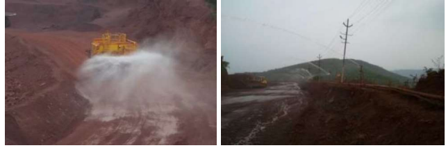
Mobile & Fixed water sprinklers in Noamundi mines
