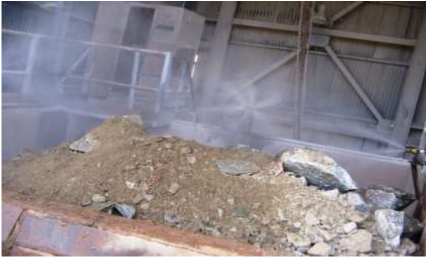
Photograph showing high pressure water spray nozzles at feed hopper
