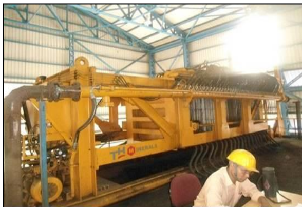
Mechanical tailings de-watering system
