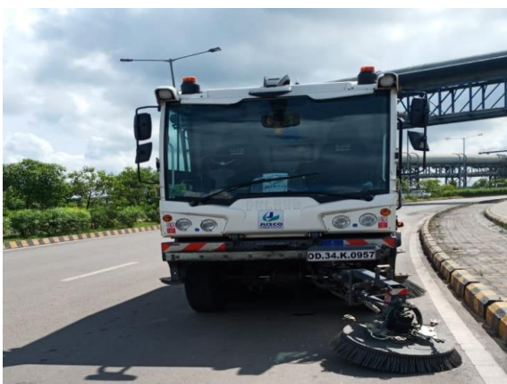
Mechanised road sweeping machine
