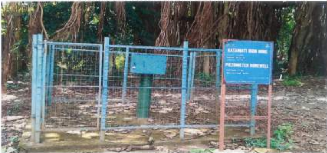
Piezometric borewell installed at Mine Office site, Katamati Mine
