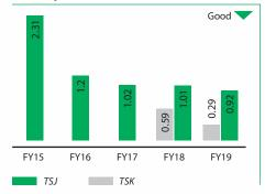
\* Specific water consumption is defined as freshwater consumption per tonnne of crude steel produced (at TSK water loss at clarifier is excluded in the calculation)
